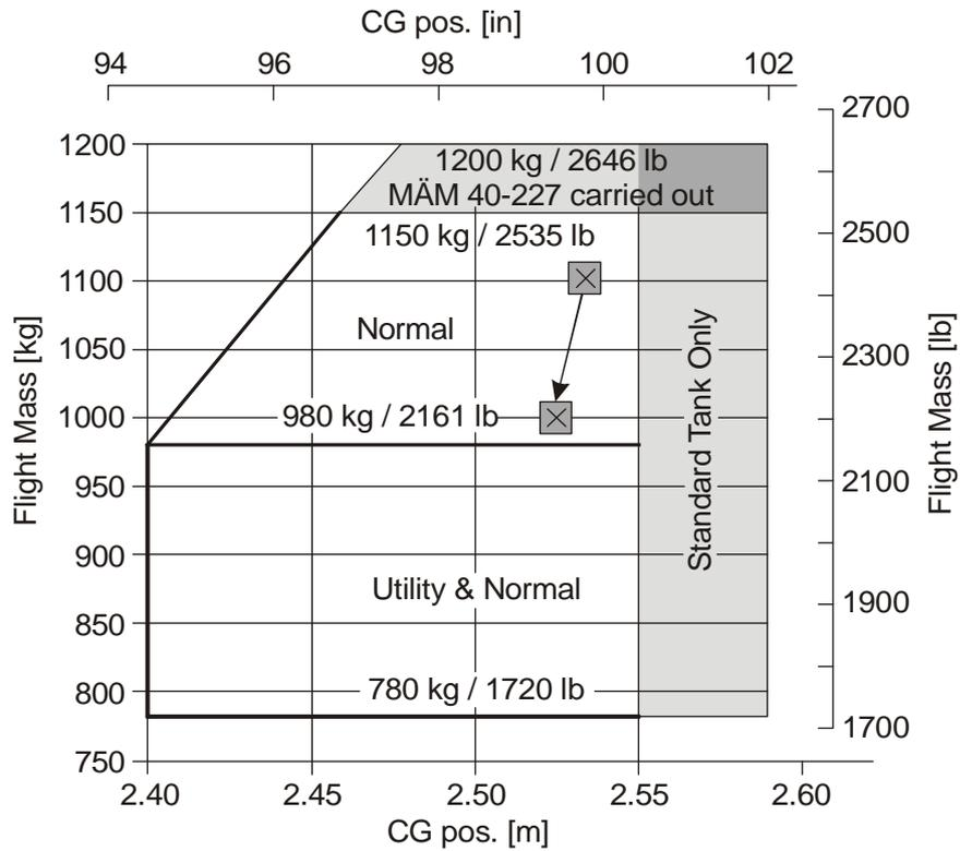
The CG's shown in the diagram are those that from the example in Table 6.4.3 - CALCULATION OF LOADING CONDITION.
