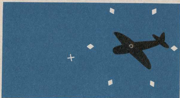
Correct—On broadside attacks the circle should be a trifle larger than length of fuselage, as wing span is greater than length.
